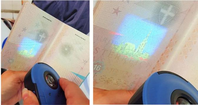
Use your thumb to press both UV light and incident light button, you start with the UV button and then let your finger slip to the incident light button to activate UV torchlight mode.
