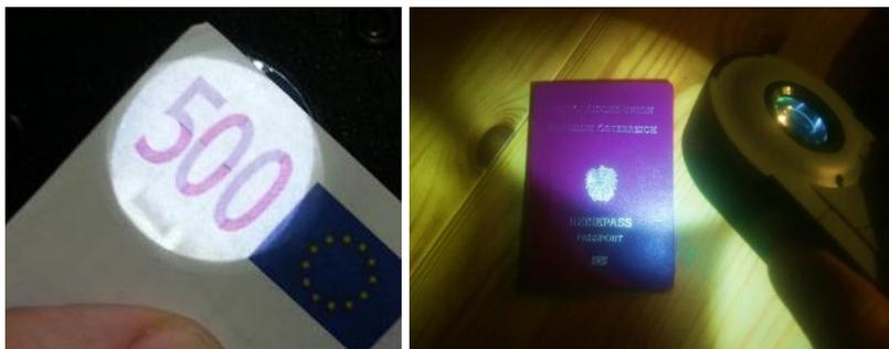
Use your thumb to press both incident light and UV light button, you start with the incident light button and then let your finger slip to the UV button to activate torchlight mode.
