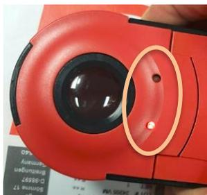
When the IR laser is activated, the red LED on the top of the device is active permanently.
