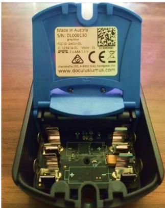
Insert the 2 AAA batteries that came with the device. Always pay attention to the correct polarity of the batteries corresponding to the markings within the device. The plus poles of the battery (marked with a +) should match the + marking near the battery clips.
